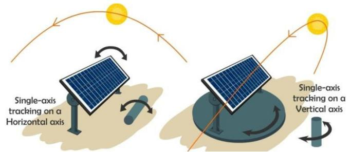
Fig 1 Solar Tracking
