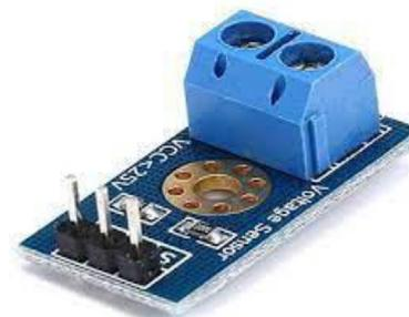
Fig 4 Voltage Sensor
